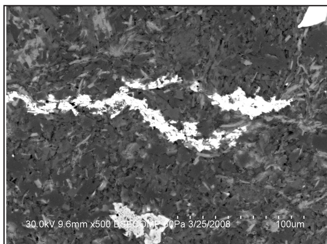
Figure 3. A dark lamina in BB-HC-A6a from the Hewitt's Cove Argillite as seen in a back-scattered electron (BSE) image acquired with a VP-SEM. The brightly contrasting minerals in the center of the photograph indicate the location of the dark lamina. EDS analysis of this layer suggests the bright minerals are allanite. This lamina contains a ring structure to the left of the photograph. The scale bar is 100 \mu\text{m} .
