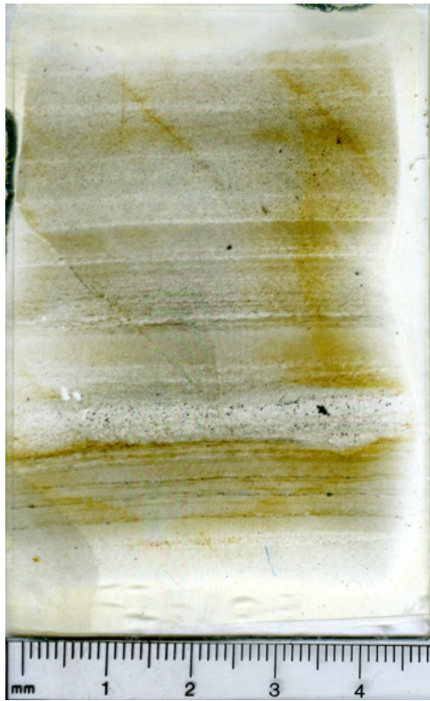
Figure 2. Large format thin section, F2b/0.9, showing finely laminated sediments ranging in thickness from 0.5 mm to 15 mm and one coarser grained laminae with a thickness of 7 mm. Grain size ranges from fine sand to fine silt. Small-scale scour mark on right side of slide.
